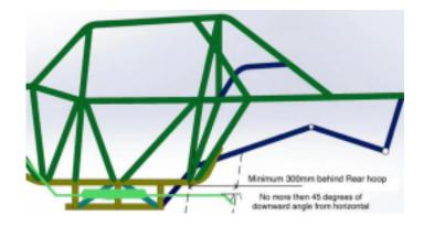
Exhausts that run to the underside of the car <u>MUST NOT</u> be pointing at the ground as to create dust. There should be no greater downward angle than 45 deg from horizontal, dust is a problem at some venues and is considered a Safety hazard. The exhaust tip at its shortest point should be no less than 300mm from the external side of the rear bulkhead. All exhausts that either exit the side or face rear and upwards must ONLY exit as a minimum 300mm from the rear bulkhead.
